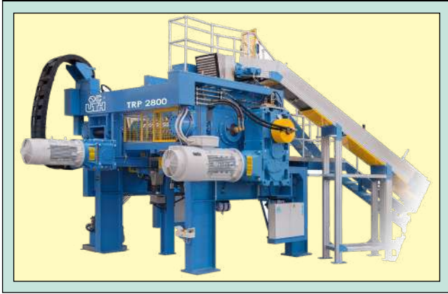
Figure 8 - TRP Reworker 2800 with integrated gear pump
