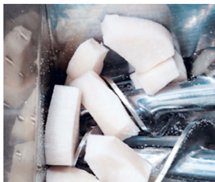
Image 1: Difficult materials or output forms can be fed in discontinuously – from left to right: polyisobutylene (PIB), butyl rubber, SBR bales
