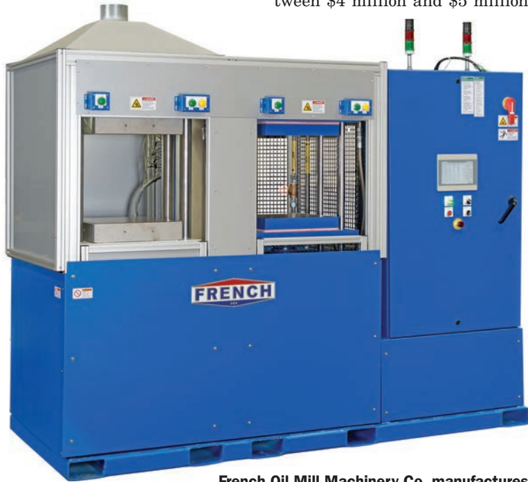
French Oil Mill Machinery Co. manufactures this 150-ton hot and cool dual press system.
