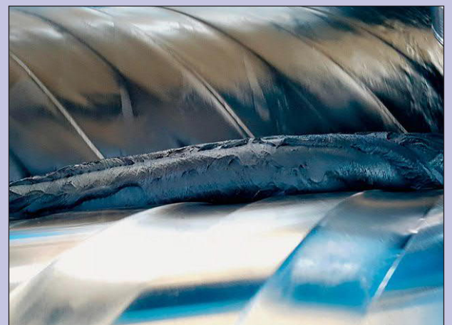
Figure 2 - homogenization of the compound on the nip of the open mill
