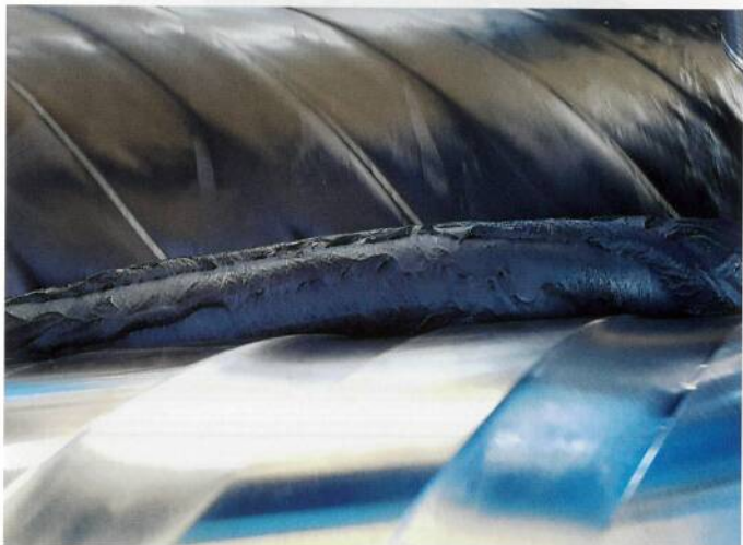
Fig. 4: Homogenisation of the compound on the nip of the open-mill
