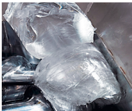
Image 1: Difficult materials or output forms can be fed in discontinuously – from left to right: polyisobutylene (PIB), butyl rubber, SBR bales
